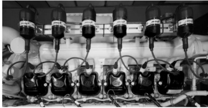
Fig. 7: Top View of a six Cylinder CHP. Upper Side of Image: Ignition Coils Mounted. Lower Side of Image: Cylinders with Spark Plugs [8].
