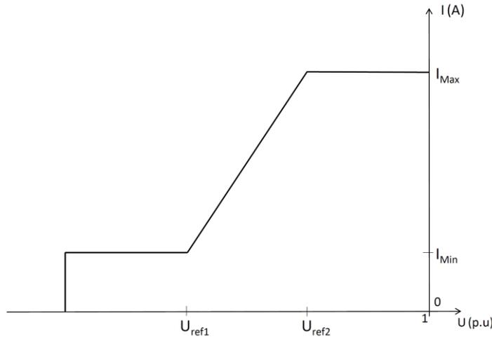
**Fig. 1.** Voltage dependent charging current characteristic curve.
