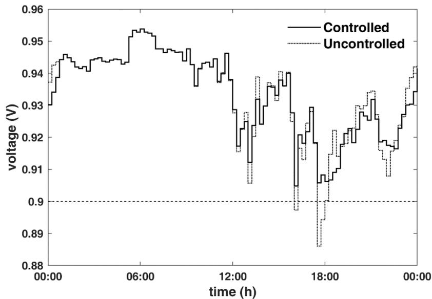
**Fig. 2.** Voltage variation at a connection node (192) with an EV.
