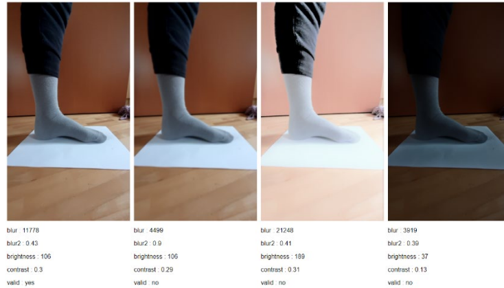
Figure 1: Images with different blur, brightness and contrast parameters. Threshold values are used to indicate the validity of the image for 3D model generation.
